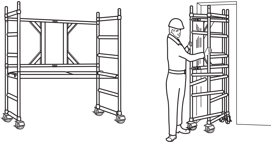
Figure 4 — Example of a room scaffold
