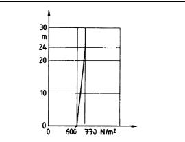
Figure 5 — Design wind pressure applying to the height above ground level
