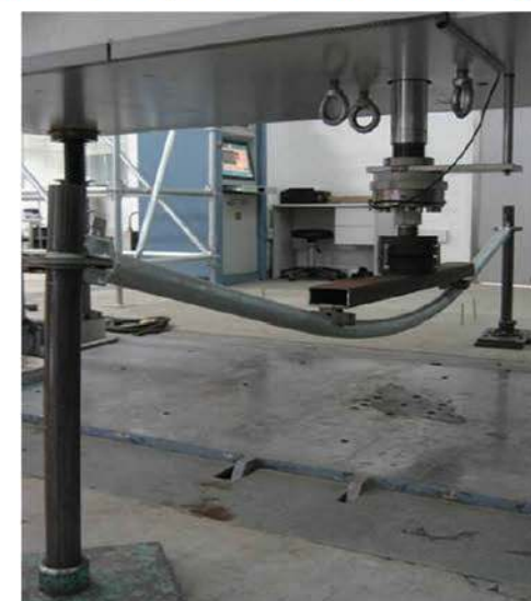
Ringlock Ledger (Load capacity test)
