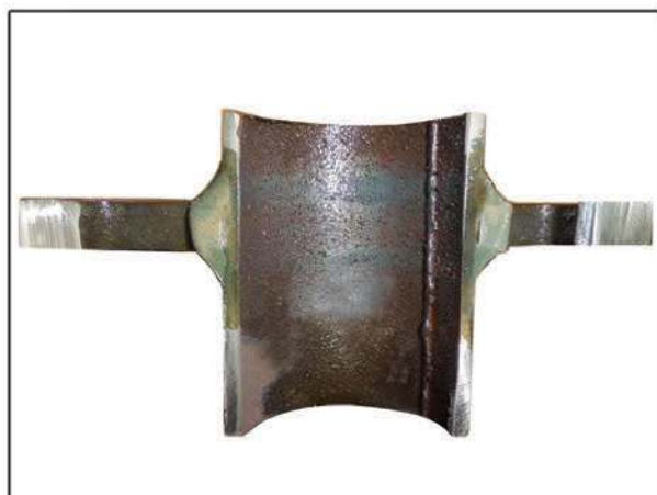
Rosette with tube welding
