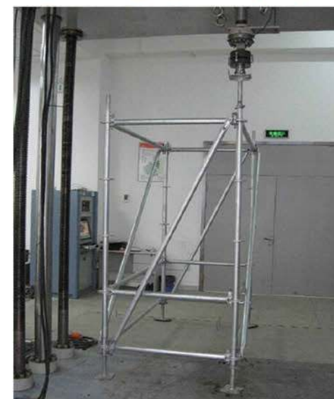
Ringlock Standard (Load capacity of single standard)
