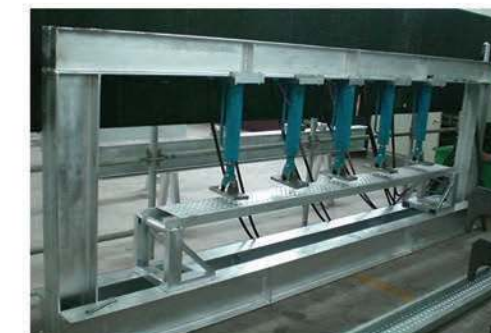
Steel Plank (Uniformly distributed load test)
