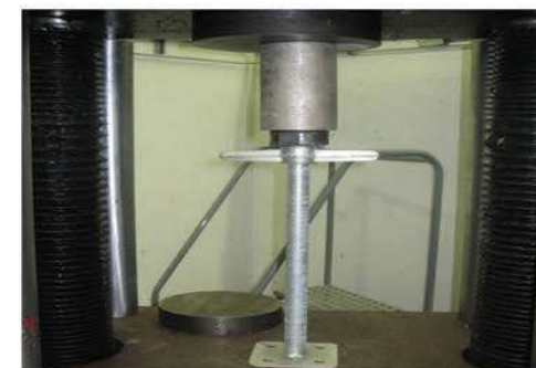
Base Jack (Test in different nut height)
